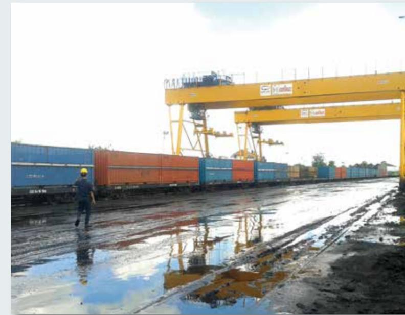
MHE-Demag supports KALOG, and Indonesia's railway sector, with portal cranes.
