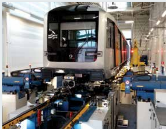
The Underfloor Wheel Lathe commissioned by MTR Corporation.
