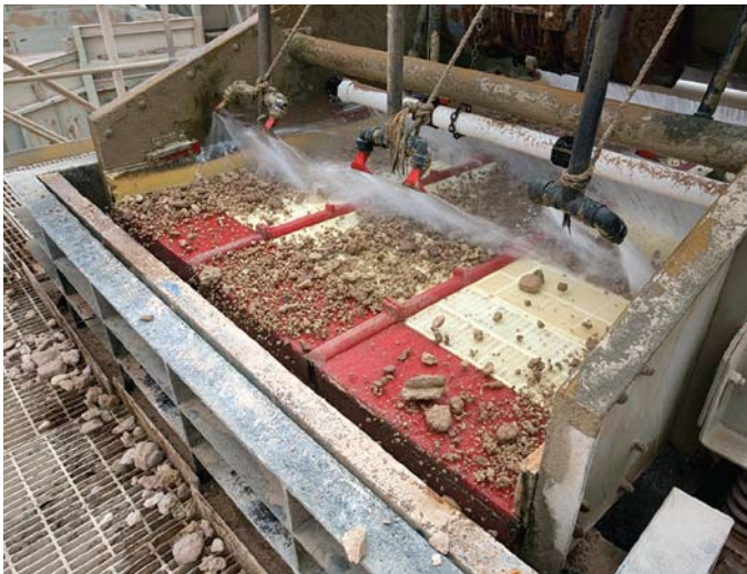
Quarry ore feed hopper trash screening to remove coarse particles before wet processing.
