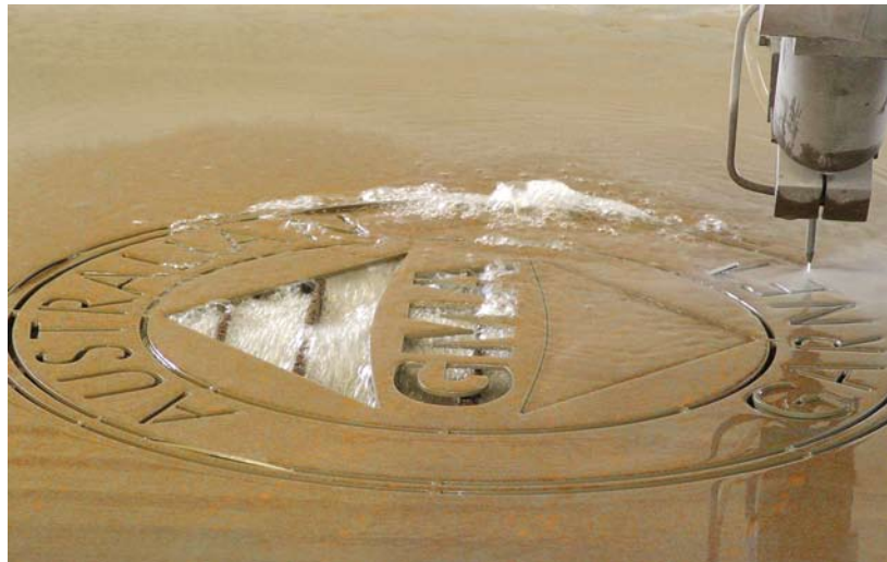
Waterjet-cutting the GMA Garnet logo in steel.
