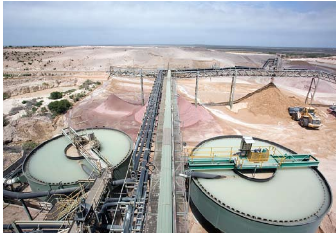
Foreground: Process water recycling and slime extraction units in the Wet Plant. Background: Piles of garnet raw concentrate (left) and sand to be trucked back to the mine backfield (right).
