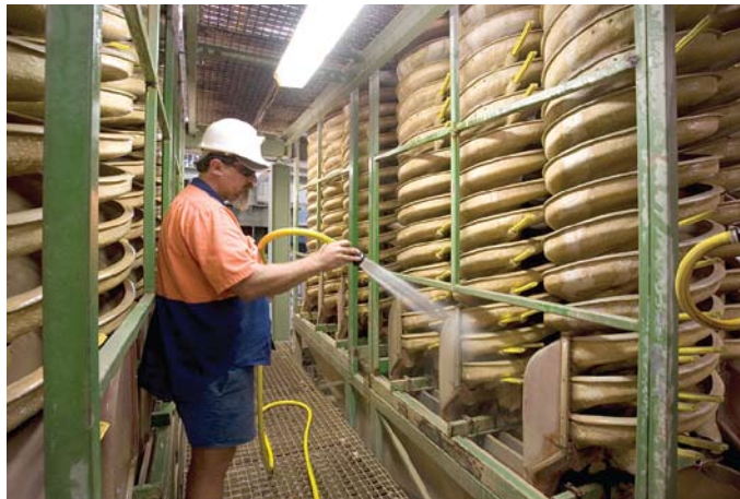
Wet processing: spiral classifiers separating garnet and ilmenite from sand.
